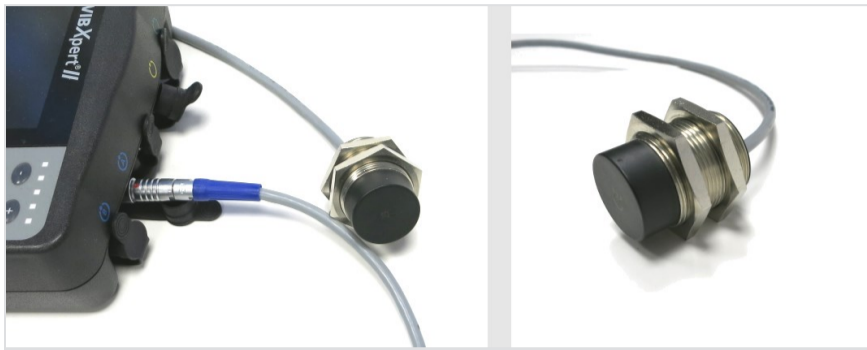
Displacement sensor connected to VIBXPERT II
