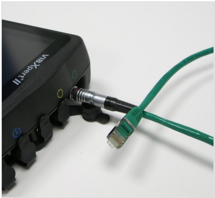
Ethernet cable connected to VIBXPERT II
